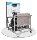
The engine is fully operational and allows the student to study diesel engine operation in starting, idle, acceleration and deceleration operating modes.
