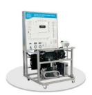
The demonstrator includes an electric motor that rotates the A/C compressor.
