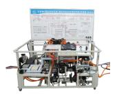
The main components are installed on the platform, including a high-voltage electronic control assembly, a BMS power battery management controller, a main controller assembly, a MICU body controller, a gateway control module, an EPB electronic parking controller and an intelligent key controller.
