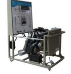
The AT-4001 Demonstrator enables actual practicing startup, speedup, slowdown and other actions of the engine.
